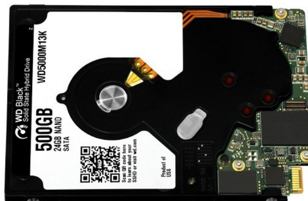
Illustration 4: SSHD Western Digital / Sandisk de 500Go (64Go de NAND)
